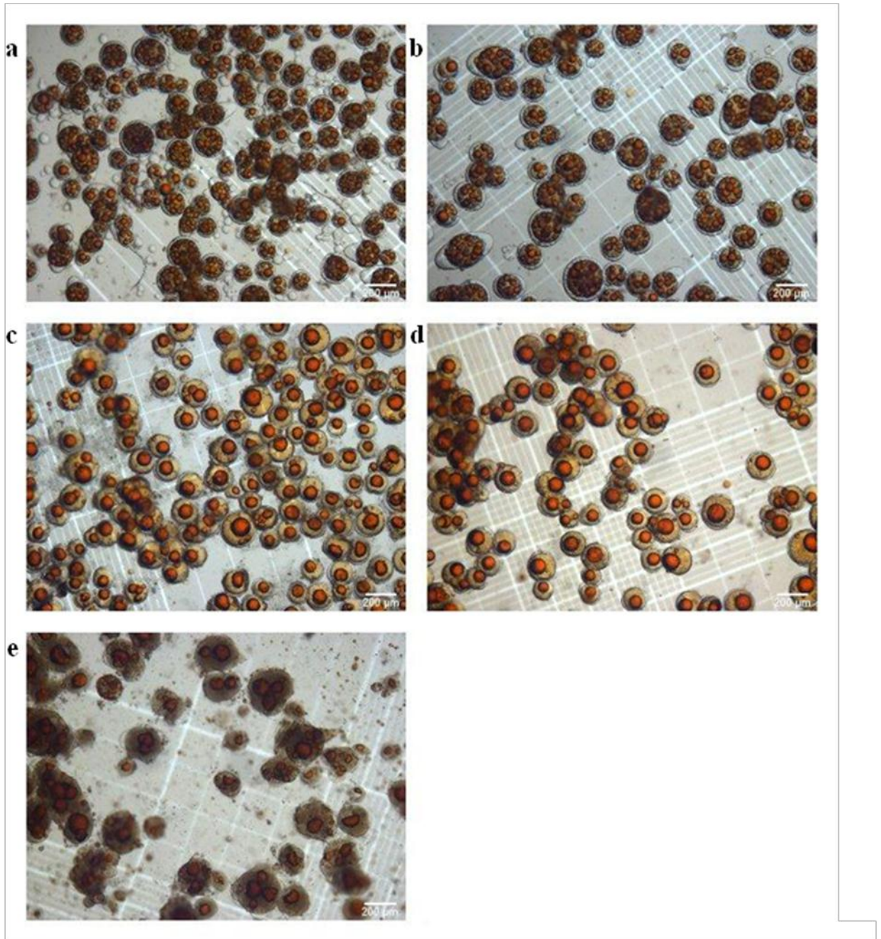
Figure 6-3. Gelatin-gum arabic coacervates observed by the stereomicroscope as a function of the ratio of the core material to the wall of (a) 1:1, (b) 1.5:1, (c) 2:1, (d) 2.5:1 and (e) 3:1. Coacervates were formed at a constant homogenization rate of 20,500 rpm, concentration of wall materials of 1%, pH of 4 and a stirring speed of 3 out of a scale of 10.
